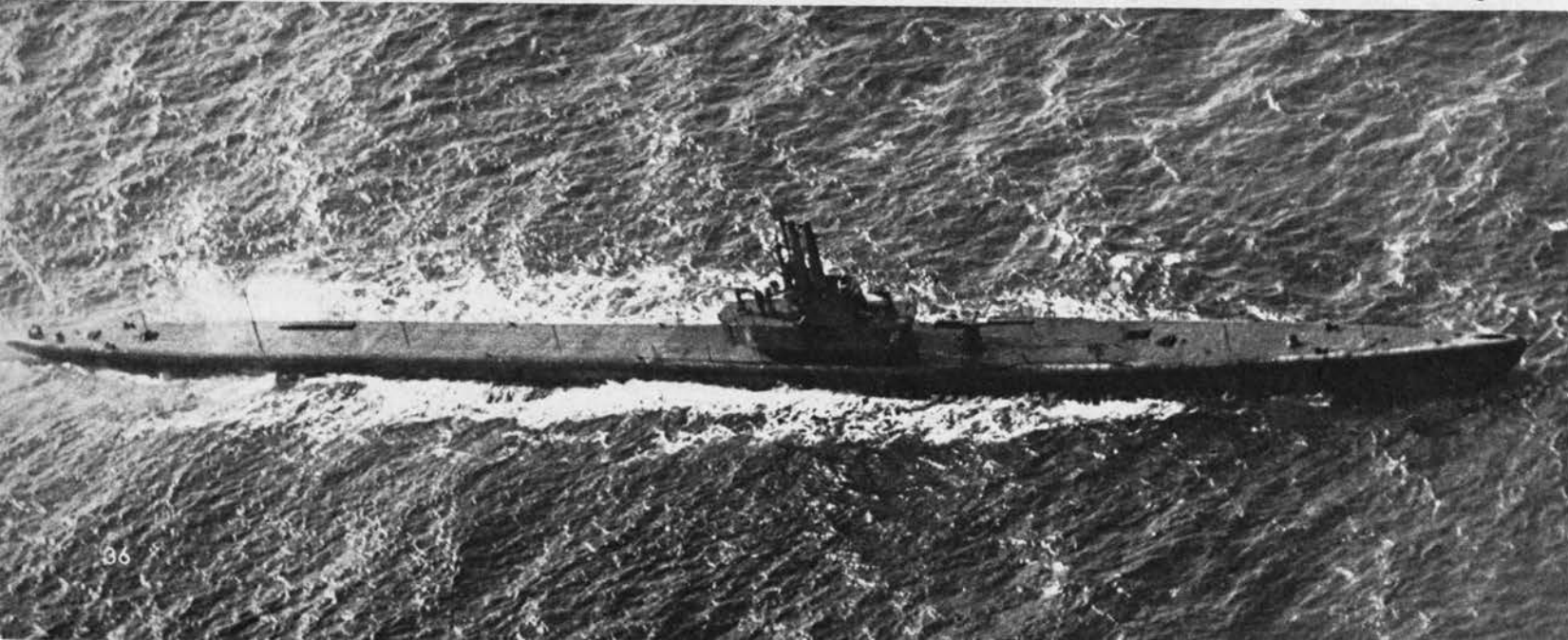
LOW, STEPPED CONNING TOWERS ARE SET WELL FORWARD ON HULLS OF U. S. SUBS. BRISTLE WITH PERISCOPE SHEARS, OTHER TECHNICAL EQUIPMENT
